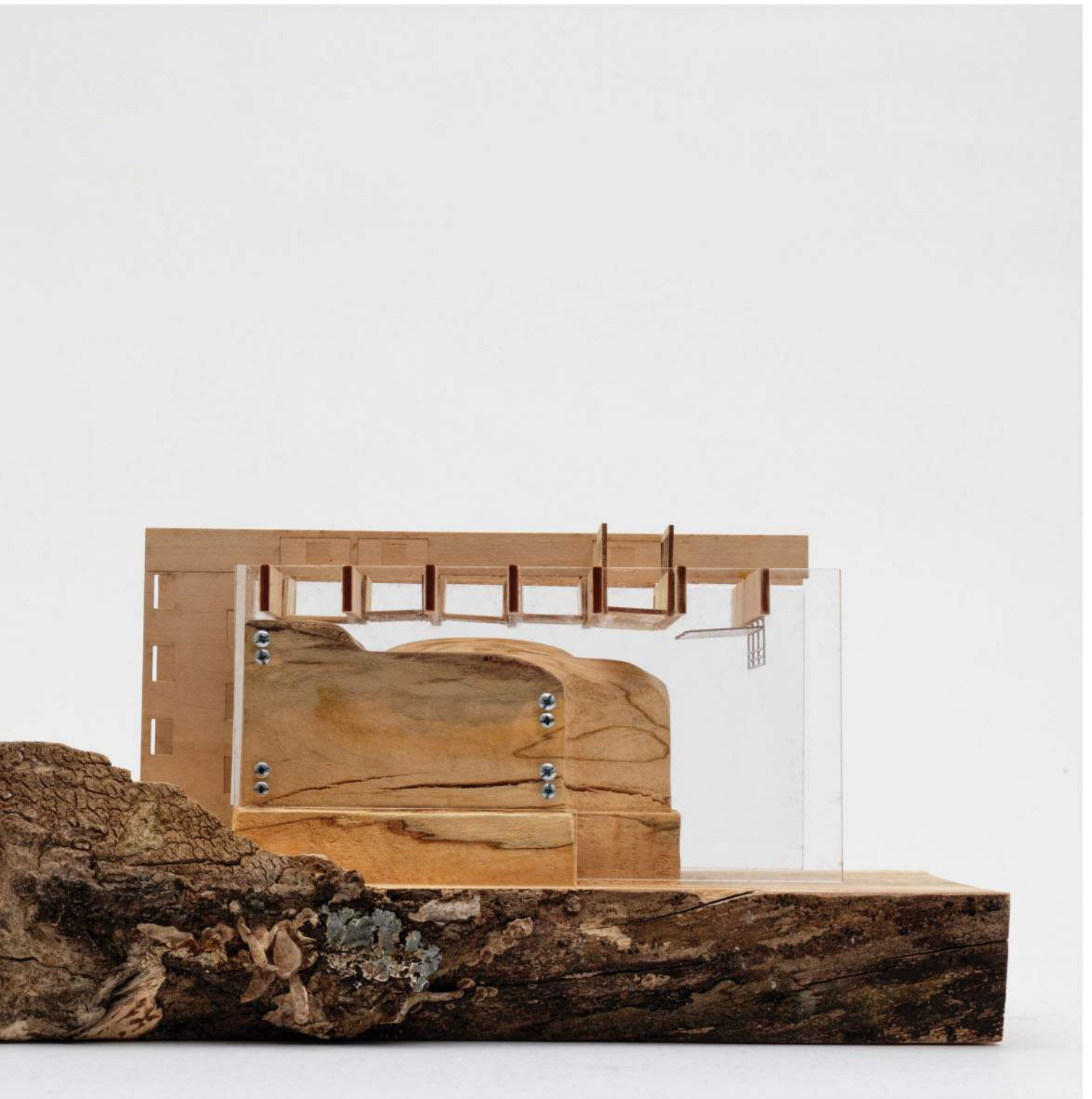
representational model, 1: 100 | using a split wood with fungal overgrowth to CNC existing theater
